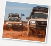
If the mud is **thick** and has a loose deep base, lower tyre pressures, avoid wheel spinning and maintain momentum.
