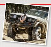
**Lower pressures** allows the tyre to improve its traction and flexibility over the obstacles without impact fracturing damage.
